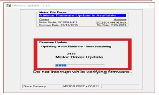
37. Now you can POWER CYCLE the motor carriage. Turn off the QuiltMotion by using the power strip switch attached to the back of the carriage. Please wait 30 seconds and then turn the power back on to the QuiltMotion and click "OK" and now turn your sewing machine back on.
