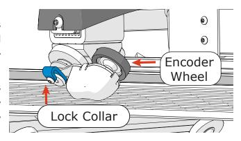
Look under the encoders to see that there is no thread or lint under or on the encoders. Check each of the encoders to make sure that they are plugged into the correct ports. Be sure to also check that all cords are plugged into the correct ports and are attached to the machine in a way that they won't get in the way.
