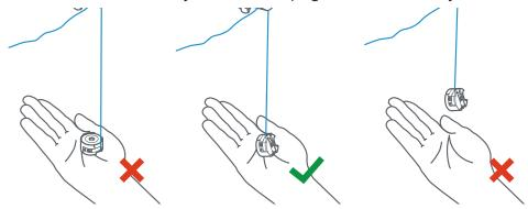
If the bobbin case remains on its side, there is too little tension. Turn the large screw (shown below in blue) clockwise. If the case lifts into the air, there is too much tension. Turn the large screw (shown below in blue) counter-clockwise.
