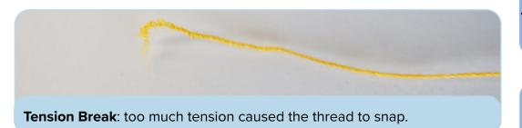
If the broken end looks shredded or coiled there may be a burr somewhere on the machine that is cutting the thread.
