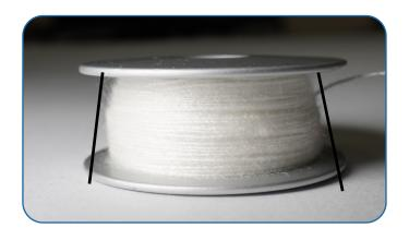
To fix coning, adjust the bobbin thread tensioner height to ensure the thread is winding at the correct angle. See your instruction manual's Bobbin Wind Troubleshooting section for instructions.
