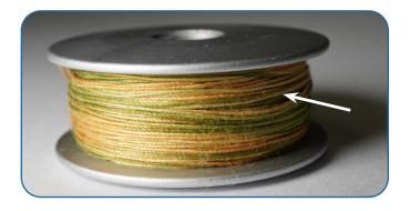
During a loose wind, stacks of the loose thread might get pinched under tighter strands or bulge out in places, creating a messy wind.
