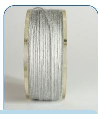
**Over-wound:** To test if your bobbin is over-wound, place it vertically on a flat surface. If one of the sides of the bobbin is lifted up then the bobbin is over-wound. Keep in mind that many pre-wound bobbins are slightly over-wound.
