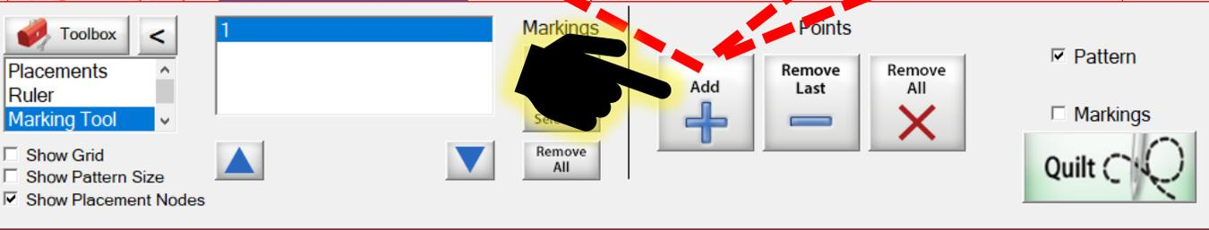
Move the machine to the outside left edge of the quilt top and tap on the “Add +” button to make a mark. (you will see a brown dot). Move the machine up to the top left corner and tap on “Add +”. Move the machine along the top edge then once again tap “Add +.” Now move to the inside edge and finish outlining the top left corner. You should finish up where you started.
